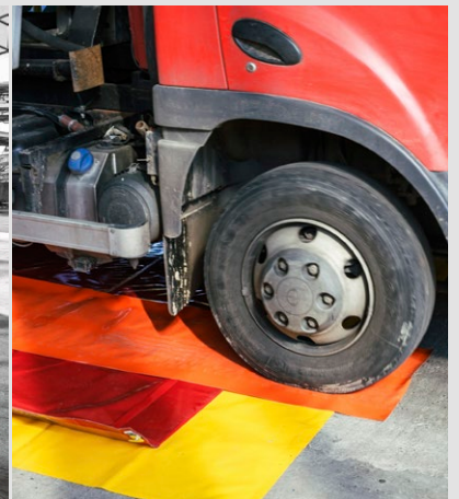
Drive in through open side wall on under-wheel tracks
